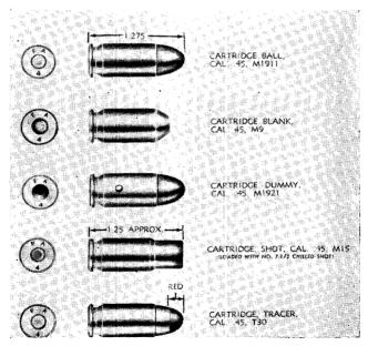
Figure 8. Caliber .45 cartridges.
