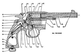
Figure 15. Revolver, Colt, caliber .45, M1917 (sectional view).
