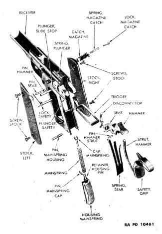
Figure 6. Receiver group of pistol, M1911A1,
