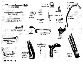
Figure 7. Group of smaller parts of pistol. M1911A1.
