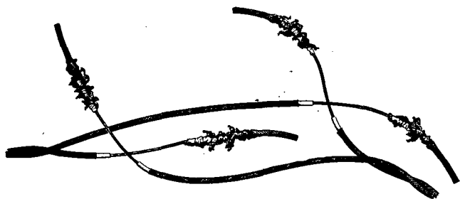
Figure 7. Wires skinned and ready for square knots.
