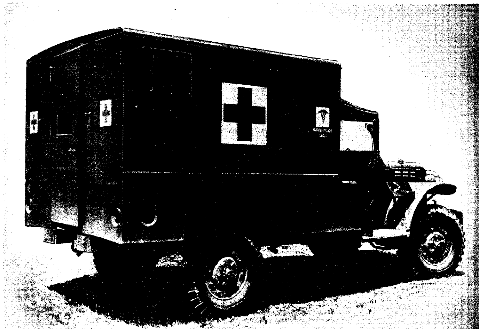
3/4-TON, 4 x 4, AMBULANCE, WITH OPEN CAB. EARLIER MODEL HAD CLOSED CAB
