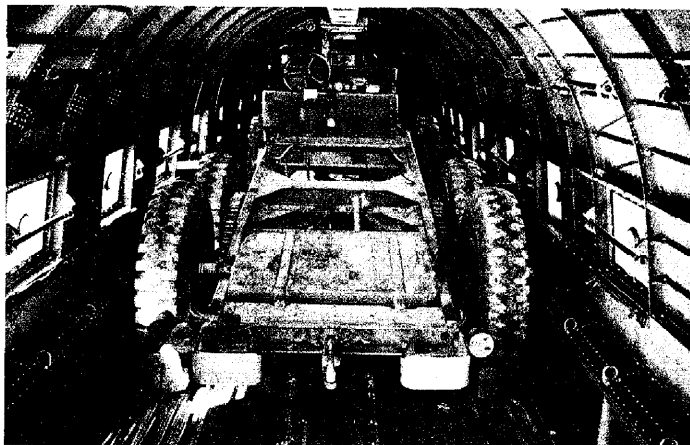
CHASSIS OF 1 1/2-TON, 6x6, TRUCK LOADED IN CARGO COMPARTMENT
