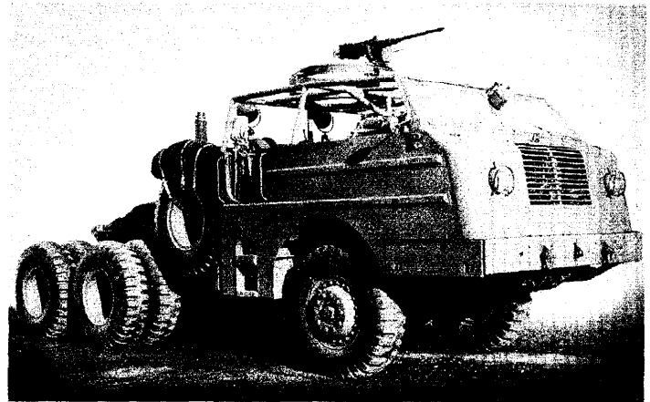
TRACTOR TRUCK M26A1 HAS UNARMORED, "SOFT TOP" CAB
