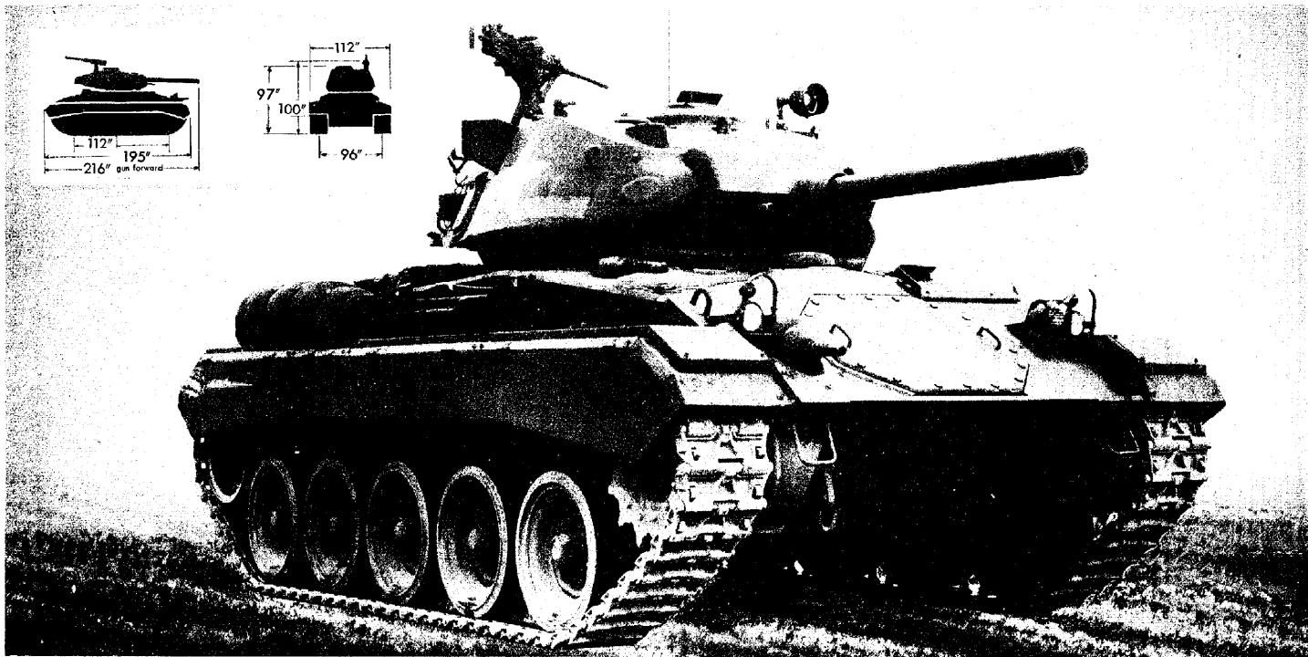
LIGHT TANK, M24, HAS LOW SILHOUETTE AND TORSION BAR SUSPENSION. IT MOUNTS 75 MM AIRCRAFT GUN IN TURRET
