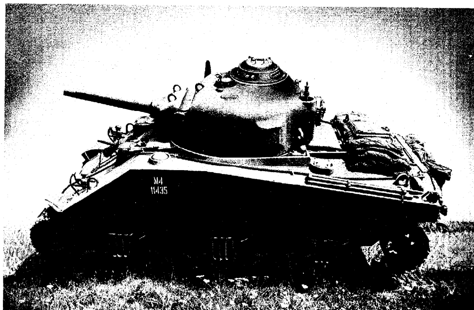
MEDIUM TANK, M4 (105 MM HOWITZER), SHOWING DETAILS OF TOP OF HULL AND TURRET
