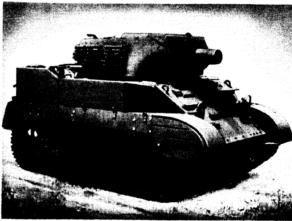
75 MM HOWITZER MOTOR CARRIAGE, M8, IS BASED ON LIGHT TANK, M5, CHASSIS
