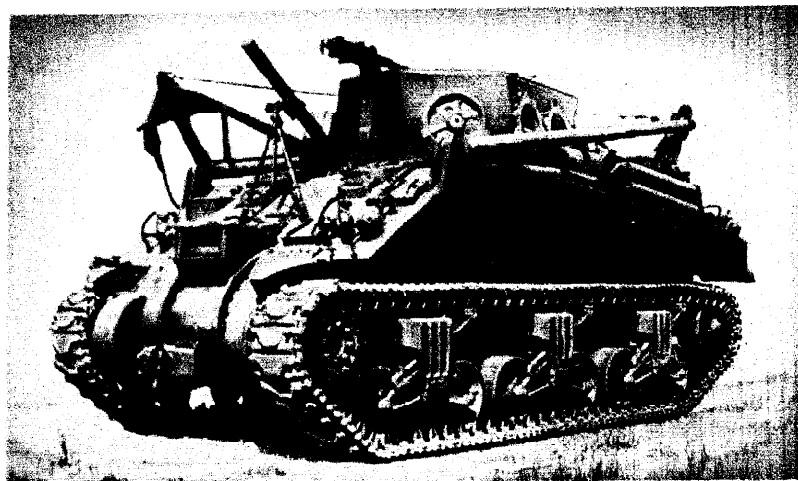
LEFT FRONT VIEW, SHOWING 81 MM MORTAR, WITH BOOM IN CARRYING POSITION
