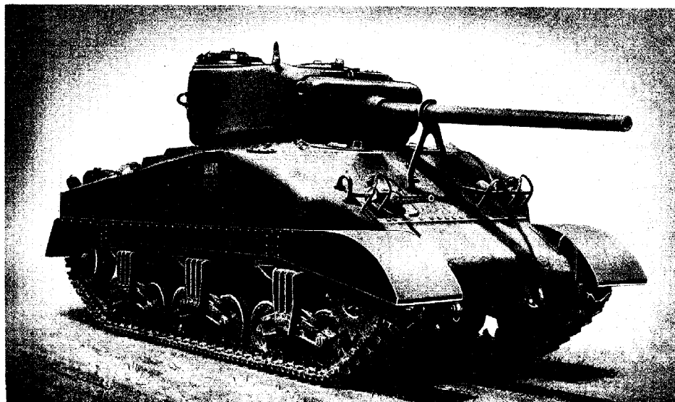
MEDIUM TANK, M4 (76 MM), WITH GUN SUPPORTED BY TRAVELING LOCK
