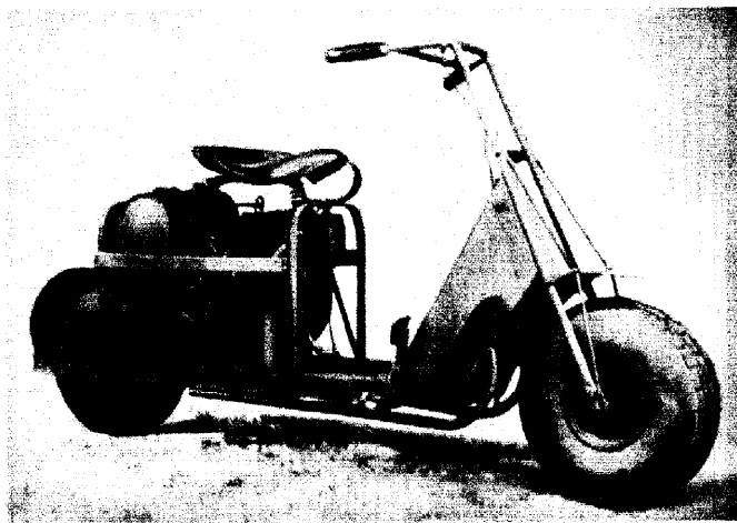
2-WHEEL MOTOR SCOOTER PROCURED FOR AIRBORNE USE
