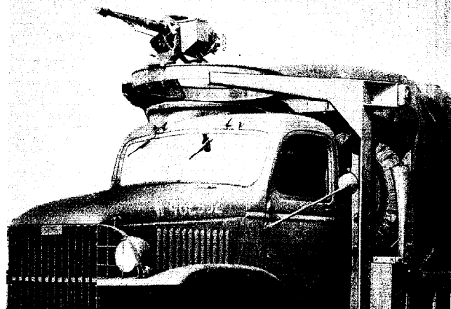
TRUCK MOUNT M37 ON SHORT WHEELBASE, CLOSED CAB TRUCK
