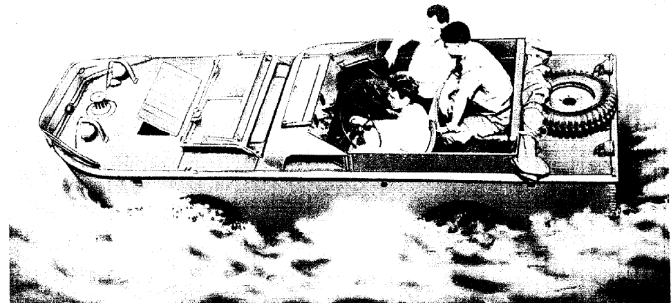
WATERPROOF HULL, PROPELLER AND RUDDER PERMIT TRAVEL IN WATER
