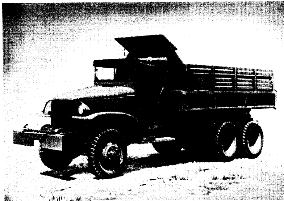
2½-TON DUMP TRUCK MAY ALSO BE USED AS CARGO AND PERSONNEL CARRIER
