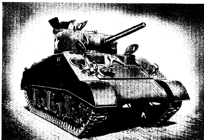
MEDIUM TANK, M4A3, WELDED, WITH CAST LOWER FRONT HULL
