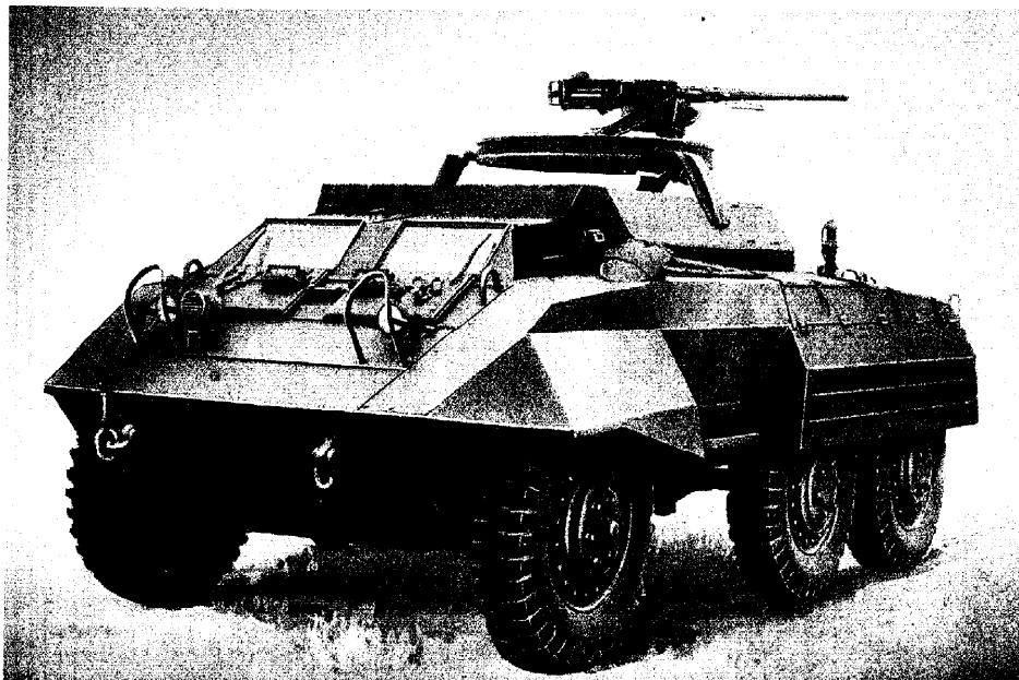
ARMORED UTILITY CAR M20, WITH RING MOUNT M49. LATER VEHICLES USE RING MOUNT M66
