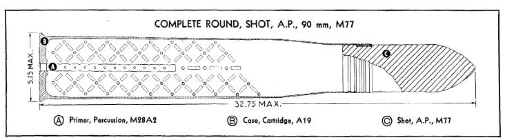
These rounds use an NH propelling charge of MI class powder with a formula of 87-10-3. The grains of this powder have seven perforations and a web of 0.049 inch.
