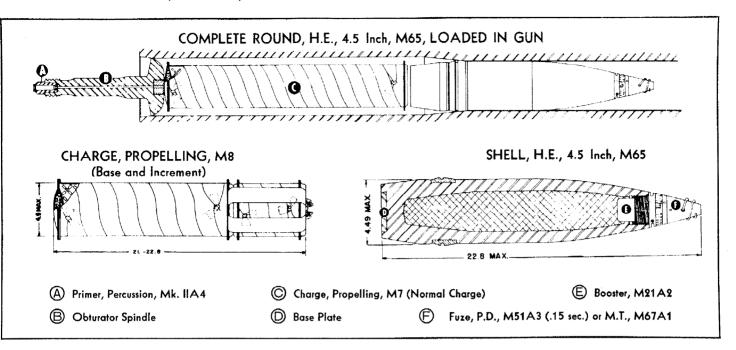
SHELL, HIGH-EXPLOSIVE, 4.5 INCH, M65, M65B1 and M65B2—STANDARD These shells are classified as standard ammunition for the 4.5 inch field gun, M1. The separate loaded complete round consists of the loaded and fuzed shell, M65, M65B1 or M65B2, with either the normal base-propelling charge, M7, or the
