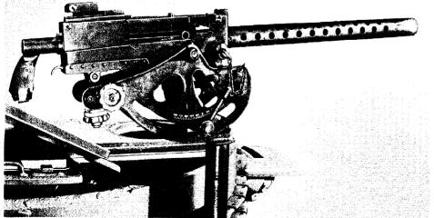
BROWNING MACHINE GUN, CAL. 30, M1919A4, IN A. A. BRACKET MOUNT ON LIGHT TANK, M5
