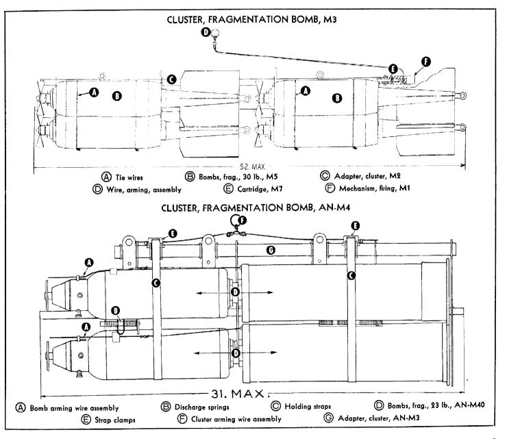
CLUSTER, FRAGMENTATION BOMB, M3—LIMITED STANDARD—The M3 cluster operates similarly to M1 and M2 clusters except that a delay cartridge is used.
