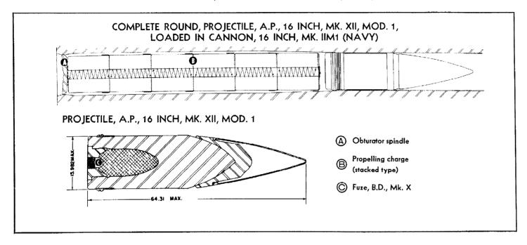
Of the projectiles that have been made for 16 inch cannon only one is now standard for issue and manufacture—the 16 inch, Mk. XII, Mod. 1. The Mk. V, the Mk. II, Mod. 2, and the Mk. IX, 16 inch, projectiles are limited standard and are only for issue until present stocks are exhausted.
