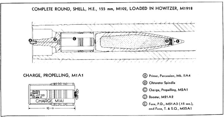
Standard ammunition for the M1, M1917, M1917A1, and M1918 howitzers is issued with high explosive or chemical fillings and with an inert filling for drill purposes. The 155 mm gun shells should not be fired in the 155 mm howitzer, as these projectiles would seat differently in the howitzer—thus reducing the chamber space for the propelling charge and giving
