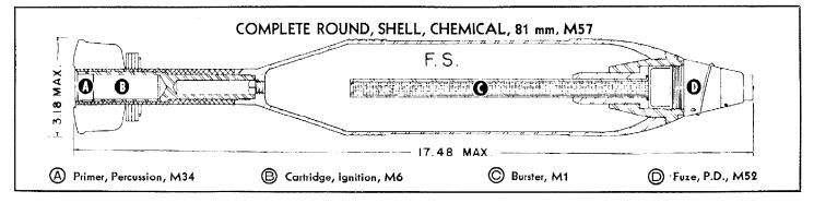
Since the last war, vast changes in design have been made in the old "Stokes" mortar projectiles to improve their ballistics and functioning.
