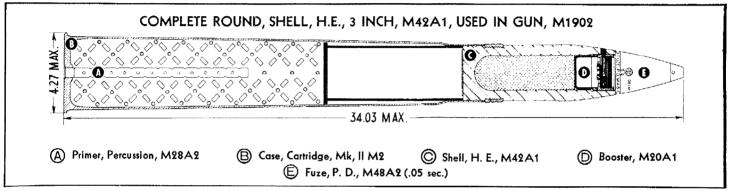
mmunition for the two models of 3 inch seacoast guns, M1902 and M1903, is still known as 3 inch "15 pounder" ammunition although the older model projectiles of that weight are no longer standard. Two types of ammunition were formerly provided for the 3 inch seacoast guns, but the high-explosive shell, M42A1, is the only standard item for issue and manufacture since the armor-piercing and high-explosive shells, M1915 and Mk. I. became obsolete.
