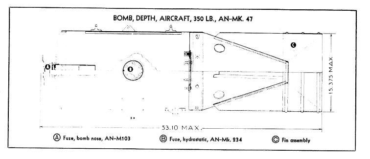
BOMB, DEPTH, AIRCRAFT, 350 LB., AN-MK. 47—STANDARD—This is the only depth bomb standard for issue and manufacture. It was originally a Navy item but has been standardized for both Army and Navy use. The AN-Mk. 47 bursting charge is torpex but a substitute standard 325 pound bomb, AN-Mk. 41, is TNT loaded.
