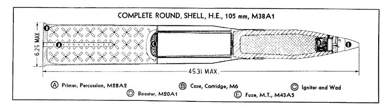
The ammunition used in the 105 mm antiaircraft gun is issued to the using arms in complete rounds of the fixed type. The round consists of a cartridge case, containing a primer and propelling charge, and a fuzed and loaded high-explosive shell.
