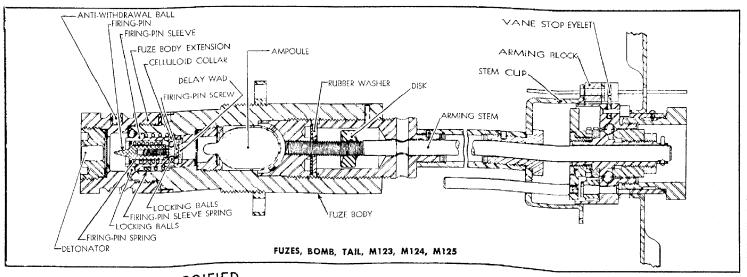
ciently into the fuze to crush a glass ampoule containing a solvent. The released solvent filters through a delay wad and attacks a celluloid collar. After a total of approximately 1,000 feet of air travel the stem has advanced sufficiently to seat a disk against a rubber washer, thus sealing the vane end of the fuze against entrance of water and leakage of solvent.
