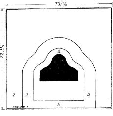
RIFLE TARGET D, 1,000 INCH-Required for firing courses A, B, C and D on the 1,000 inch range with cal. .30, M1903 and M1, rifles. Printed in black on buff manila target paper 12 inches square. Packed 1,000 in a package, each package wrapped completely and securely in paper with label pasted on outside indicating contents.
