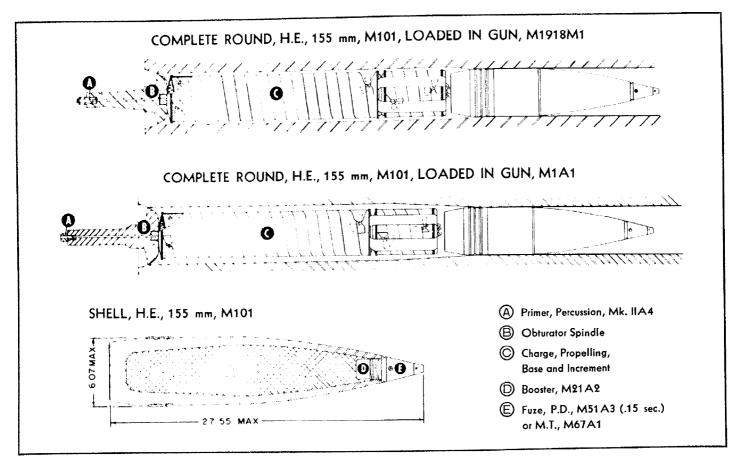
The 155 mm guns, M1917, M1918M1, M1 and M1A1, take the same separateloading projectiles. Loading is accomplished in three operations: (1) inserting the projectile in the gun, (2) inserting the propelling charge and (3) inserting the primer in the breech mechanism of
