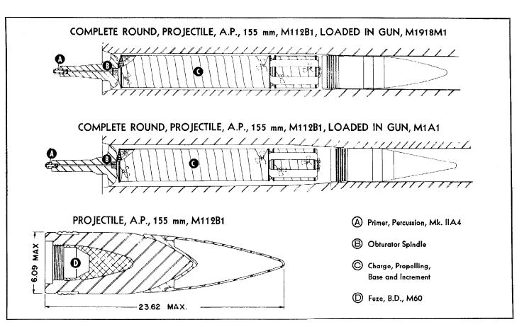
PROJECTILE, ARMOR-PIERCING, 155 mm, M112B1—STANDARD—The projectile measures 23.62 inches in length over-all, and as fired weighs 100 pounds. It contains 1.44 pounds of explosive "D" bursting charge which is detonated by fuze, B.D., M60. In the M1918M1 gun, the projectile is propelled by a base and increment charge of 24.75 pounds of NH powder. This provides a muzzle velocity of 2,360 feet per second and a maximum
