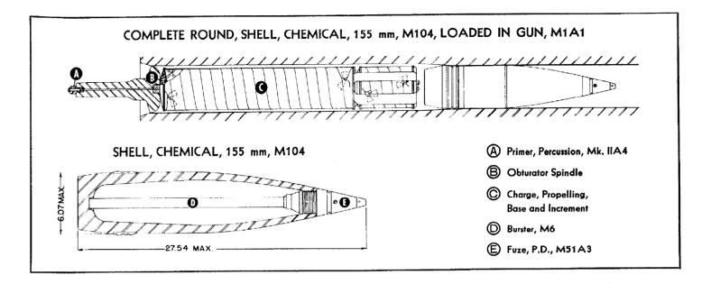
SHELL, CHEMICAL, 155 mm, M104-STANDARD—This is a standard issue and manufacture round for use in the M1 and M1A1 guns and consists of the chemical shell, M104, with burster, M6, booster, M22, and fuze, P.D., M51A3. The shell measures 27.54 inches in length.
