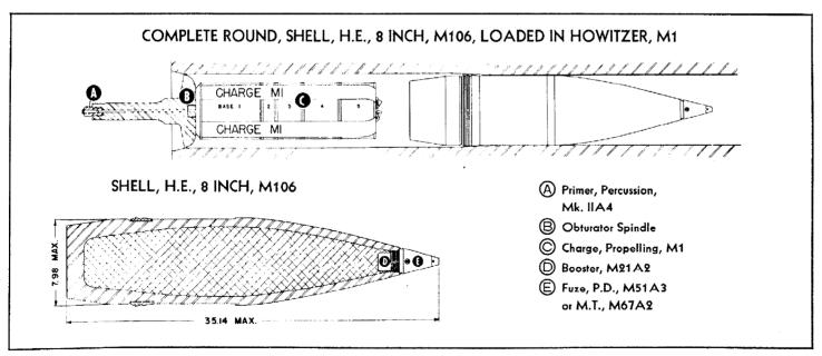
The Mk. I high-explosive shell used in the 8 inch guns was modified to take either the point-detonating fuze, M51A3, or the mechanical time fuze, M67A2. This modification was designated high-explosive shell, Mk. IA1, and is used in the M1 howitzer.
