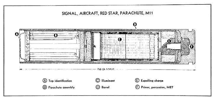
SIGNAL, AIRCRAFT, RED STAR, PARACHUTE, M11—STANDARD—This item is the only remaining standard parachute aircraft signal for issue and manufacture since the M14, red star, cluster; M15, white star, blinker; and M16, green star, blinker, signals were classified limited standard.
