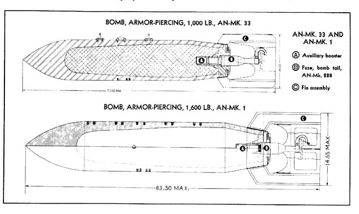
BOMB, ARMOR-PIERCING, 1,000 LB., AN-MK. 33—STANDARD—The complete round assembly of this bomb consists of: Romb A. P. 1,000 lb AN.Mb 33
