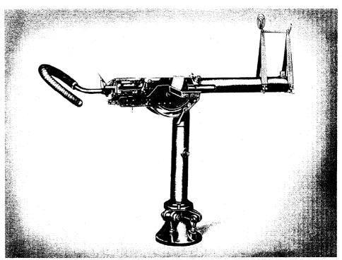
MOUNT, MACHINE GUN, CAL. .50, A.A., M2A1, ON PEDESTAL BASE
