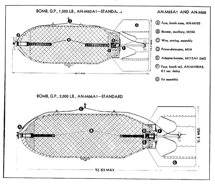
The large general purpose bombs are used against reinforced concrete bridges, clams, steel railroad bridges, piers, approach spans, such seacraft as heavy cruisers, etc.
