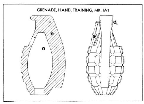
GRENADE, HAND, TRAINING, MK. IA1—STANDARD—This grenade is the current standard for practice and training. It consists of a one piece cast-iron body in the shape of a Mk. II fuzed fragmentation grenade and a removable safety pin and ring. It is inert. The grenade weighs 22 ounces, 1 ounce more than the Mk. II.
