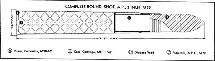
Due to the additional manufacturing steps necessary in the production of the three-piece M62A1 projectile, the easily made 3 inch monobloc projectile,
