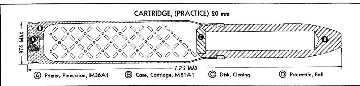
he armor-piercing, shot, M75, and ball projectile (practice) are standard ammunition and are turned out of steel bar stock instead of being forged or cast. The propelling charges used with these cartridges are made from IMR powder of single-perforated grains with a 0.021 inch web.
