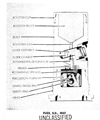
This fuze incorporates a plunger assembly of the Semple centrifu plunger type. The firing-pin is mounted in the percussion plunger a rotor which is held in the unarmed position by two safety-p which compress their springs and move out of the rotor when shell attains sufficient rotating speed. The rotor is then free to trand the pin snaps into the armed position, where it is held aw from the primer by two restraining springs.
