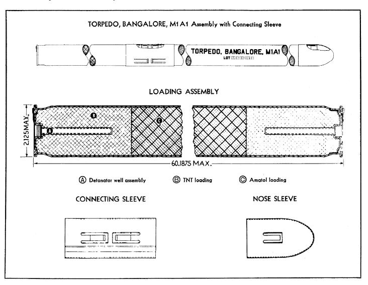
TORPEDO, BANGALORE, M1A1—STANDARD—The Bangalore torpedo is a tube filled with high explosive and used primarily for blasting an opening through wire entanglements and for clearing mine fields. The M1A1 Bangalore torpedo consists of a steel tube, 5 feet long and 21/8 inches in diameter, flanged and capped at each end.
