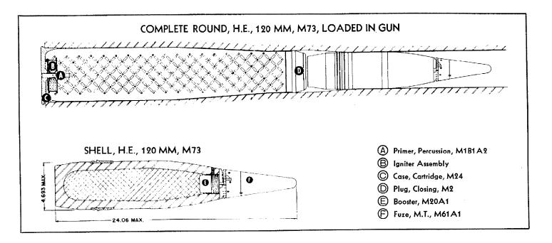
SHELL, HIGH-EXPLOSIVE, 120 MM, M73—STANDARD—This shell is standard ammunition for the 120 MM antiaircraft gun, M1.
