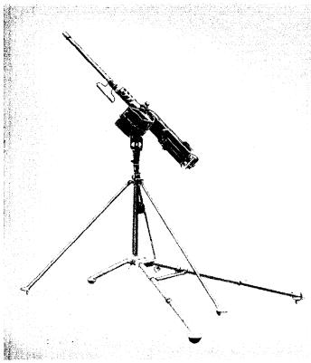
ELEVATOR-CRADLE, A.A., CAL. .50, MT, WITH GUN IN POSITION
