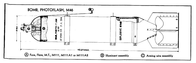
The complete round consists of the Bomb, Photoflash, M46, unfuzed, adapted for Nose Fuze, M111; Fuze, Flare, Mechanical Time, M111, M111A1 or MI 111A2 sealed; Arming Wire assembly, **Piece** mark 82-3-234GB.
