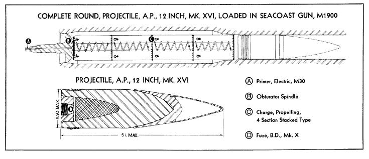
The 12 inch separate loading ammunition is used in the 12 inch seacoast guns M1888, M1888MI, M1888MII, M1895, M1895MI and M1900.
