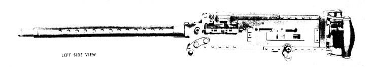
BROWNING MACHINE GUN, AIRCRAFT, CAL. .30, M2, FLEXIBLE-LEFT HAND FEED
