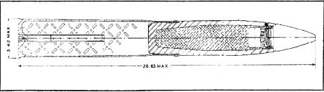
The normal charge gives a muzzle velocity of 1,470 f/s and a pressure of 26,000 p.s.i.
