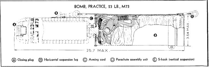
BOMBS, PRACTICE, 23 LB., M71 AND M73—STANDARD—Due to the fact that the 17 pound practice bomb, M37, could be used only in aircraft where vertical suspension was available (and therefore could not be used for clustering), the M71 and M73 practice bombs were standardized.
