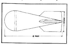
SIGNAL, DRIFT, DAY, AN-MK. I—STANDARD—This signal consists of a streamlined paper shell containing a metallic powder and is used as a daytime reference point for aerial navigation when dropped on the water. The shell breaks open upon impact and the metallic contents of the tube form a bronze slick on
