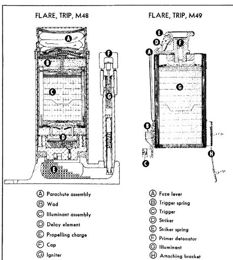
the illuminant shell to an altitude of approximately 250 to 400 feet. The propelling charge also activates a threesecond delay fuze which at the end of the delay time ejects the illuminant assembly, similar to that of the Shell, illuminant, 60 mm, M83. The illuminant burns for about 20 seconds while drifting earthward attached to a parachute. The flare burns with approximately 110,000 candlepower. The effective illumination is designed to cover a radius of 300 yards.
