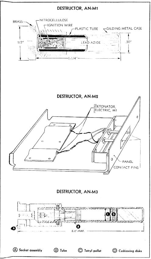
The Destructors, AN-M1, AN-M2, and AN-M3, are electrically fired explosive charges used for the destruction of radio equipment and other confidential materiel to obviate the danger of this equipment being captured by the enemy. Fittings and adapters hold the destructors in place in the materiel and provide electrical circuits and connections through which a minimum voltage of 6 volts may be passed.
