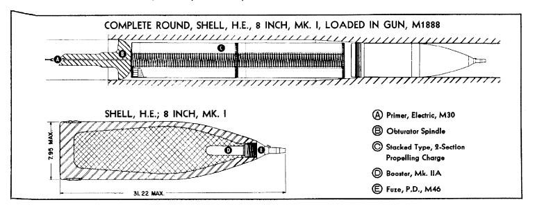
SHELL, HIGH-EXPLOSIVE, 8 INCH, MK. I—STANDARD—The Mk. I round is used in the M1888, M1888MI and MI 1888MII guns. As fired, the shell weighs 200 pounds and contains a bursting charge of 29.6 pounds of TNT which is detonated by the fuze, P.D., M46, or P.D., M47, with the Mk. IIA booster.
