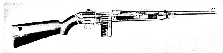
PHANTOM VIEW OF U. S. CARBINE, CAL. .30, M1, from Which U. S. Carbine, M1A2, Differs Only in Employing an Aperture Type Rear Sight Instead of an L-Type Rear Sight
