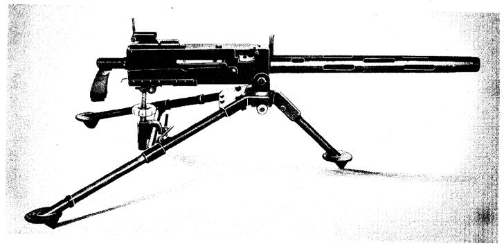
BROWNING MACHINE GUN, CAL. .30, M1919A4, ON TRIPOD MOUNT, M2
