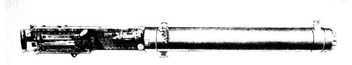
BROWNING MACHINE GUN, CAL. .50, M2, WATER-COOLED, FLEXIBLE
