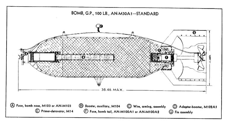
The general purpose bomb is used for destruction or demolition of matériel targets, the destructive effect being produced by the blast of the detonation. If the detonation occurs above the ground, additional damage will be caused by fragments of the bomb.
