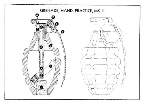
GRENADE, HAND, PRACTICE, MK. II—STANDARD—This is a standard practice grenade and is equipped with the igniting fuze, M10A3. The grenade is loaded with a small charge of black powder in a cloth bag.
