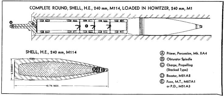
The projectiles provided for use in the 240 mm howitzers, M1918M1 and M1 are of three types: high-explosive-for use against personnel and structures; target-practice-sand loaded; and dummy —for drill purposes.
