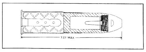
tice shell when loaded and fuzed weighs 1.63 pounds and is propelled by .056 pound of FNH powder which is ignited
