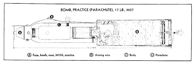
BOMB, PRACTICE (PARACHUTE), 17 LB., M37 — LIMITED STANDARD — The complete round assembly consists of the following components:
