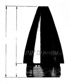
FUZES, DUMMY, M50, STANDARD— M50B1, M50B2, ALTERNATES
