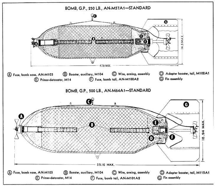
STANDARD—This bomb is particularly effective when used against railroad equipment and trackage, railroad terminals and similarly constructed buildings, ammunition dumps and seacraft such as submarines, transports, destroyers, etc.
