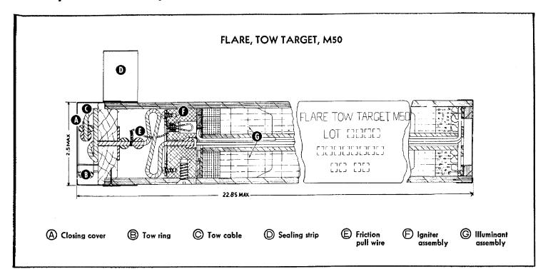
FLARE, TOW TARGET, M50—STAND—ARD—Flare, tow target, M50, provides a target for both night and day practice firing of antiaircraftguns. The flare is towed by a plane at the end of a steel cable. When one flare burns out, another may be released from the plane to take its place. The flare is not so bright that it will obscure the navigation lights of the plane, or that it will require the use of filters in fire control instruments.
