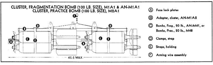
The assembly of bombs in clusters permits a large number of small bombs to be carried in stations designed for larger bombs. In operations, the release of bombs from cluster assemblies is equivalent to salvo bombing.
