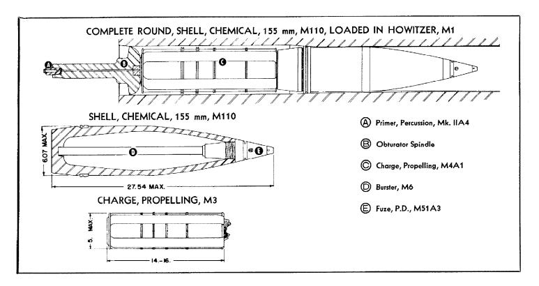
SHELL, CHEMICAL, 155 mm, M110— STANDARD—The M110 chemical shell uses the M6 burster and the fuze, P.D., M51A3 with the M21A2 booster.
