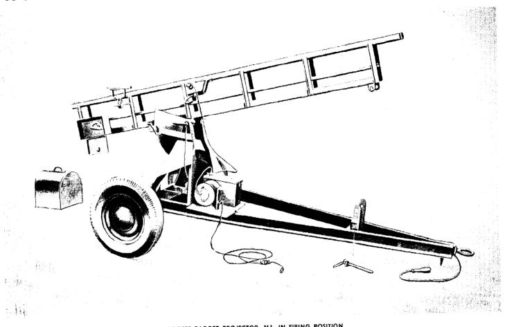
ROCKET TARGET PROJECTOR, M1, IN FIRING POSITION
