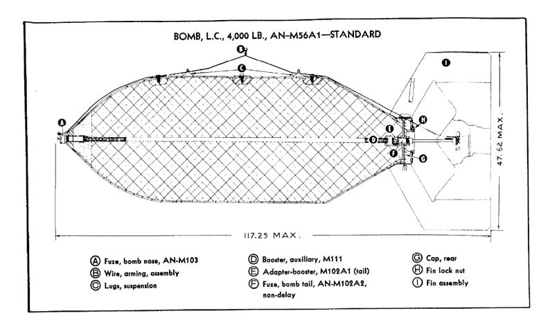
STANDARD—This is one of the heaviest bombs manufactured, and is known as the "block buster." Its large explosive charge and thin wall case make it effective against buildings and naval targets. It depends upon its blast effect for the mount of damage. The fact that very little metal, in relation to the total weight, is used places the bomb in the light case class with the explosive filler approximating 77% of the total weight.
