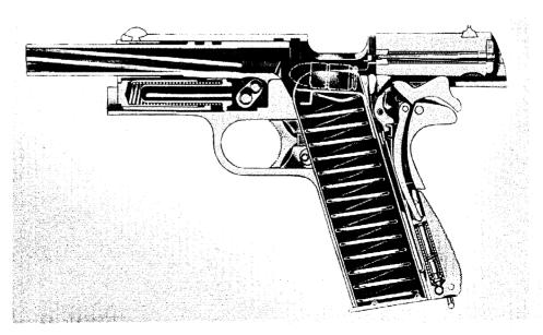
AUTOMATIC PISTOL, CAL. .45, M1911A1, SECTIONAL VIEW
