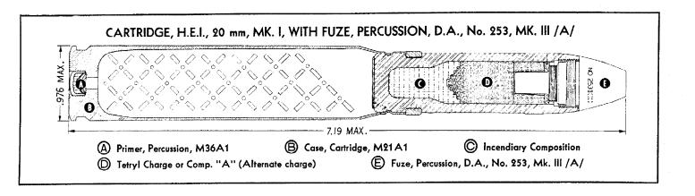
SHELL, HIGH-EXPLOSIVE INCENDI-ARY, 20 mm, Mk. I-STANDARD-This shell for the 20 mm automatic guns, M1. AN-M2, and British Hispano-Suiza /A/, was adopted from the British early in 1941 and standardized in August of that year. There have been few changes except in the redesign of the cartridge case and primer.
