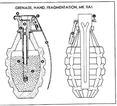
GRENADE, HAND, FRAGMENTA-TION, MK. IIA1—STANDARD—The body of this grenade is made of cast-iron and is about the size of a large lemon. The outside surface is deeply serrated horizontally and vertically to assist in producing uniform fragments when the grenade explodes. The bursting charge is 0.74 ounce of EC Blank Fire Powder initiated by the M10A3 igniting fuze.
