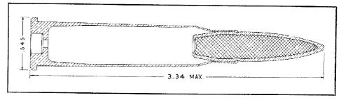
dimensions, the ammunition regularly used with the gun. To the base of the subcaliber cartridge case are fitted two flat steel extractor springs, secured by one screw each, which serve to eject the subcaliber ammunition.
