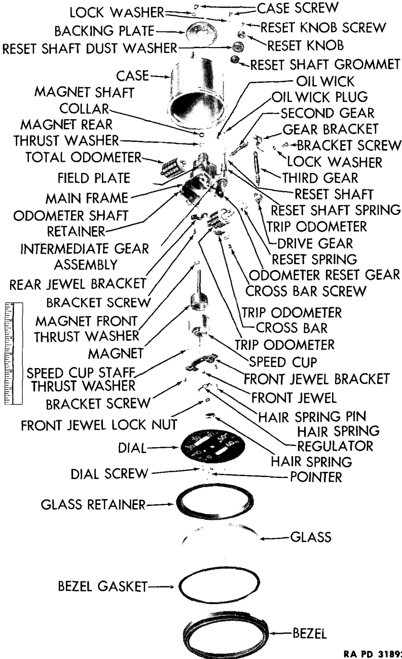
Figure 50—Stewart-Warner Speedometer with Cup-type Magnet Disassembled
